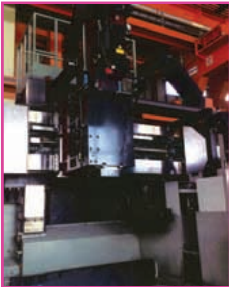
Machine without guards ready for testing and alignment checks.
